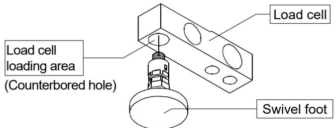
Screw the swivel foot into the counterbored hole as far as it will go, then using a wrench on the cup, tighten additionally.
