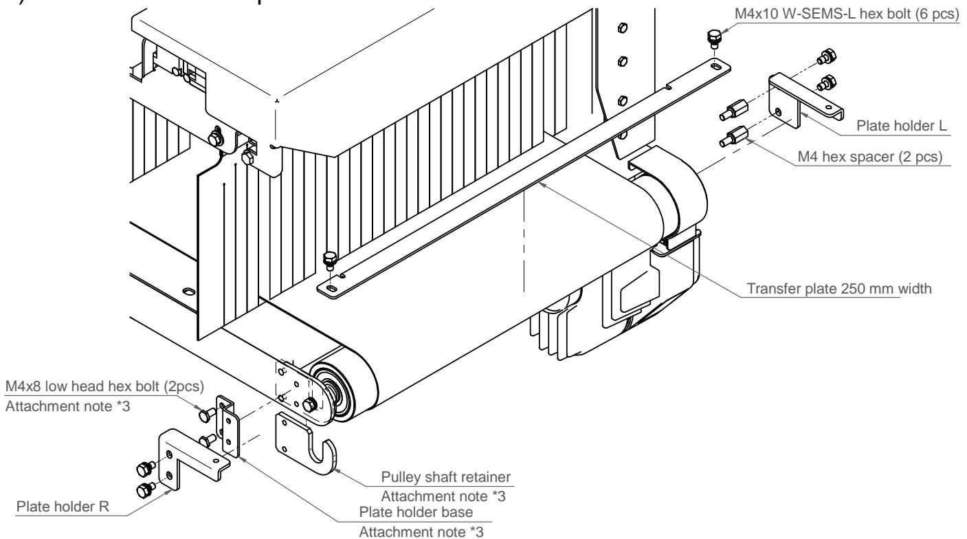
\*3: Attach the low head hex bolt while pressing the pulley shaft retainer against the shaft of the pulley.
