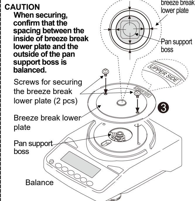
**CAUTION** - When installing, use care not to apply excessive load to the sensor mechanism (circumference of the pan support boss) of the balance.
