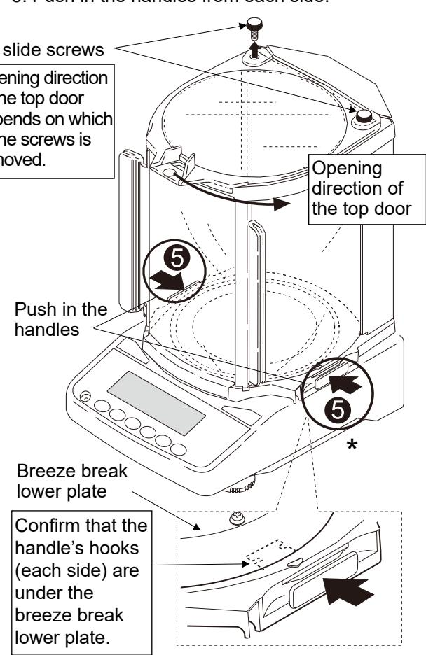
\* When used with FZ-WP / FX-WP the breeze break cannot be secured on the balance whether the handles are pulled out or pushed in.
