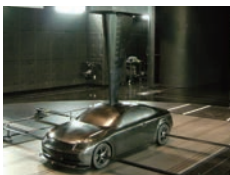
Moving floor belt system for large wind tunnels made for Nissan Motor Co., Ltd.
