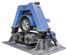
Belt testing machine for small tires made for Nagoya University
