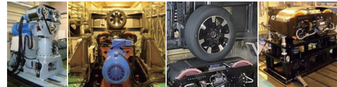
Example use with moving belt unit with vibration function for vertical and steering directions
