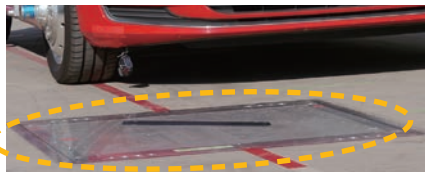
3 component force sensor with cleats buried in road surface
